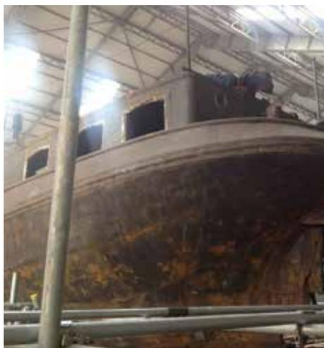
would be rebuilt, and strengthening sections welded into place to protect some of the plate joints where rivets had completely rotted away.
